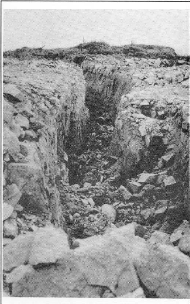
3. (left) A lead rake exposed by stripping for fluorspar on the north end of the Crich anticline, 24th October 1970.
