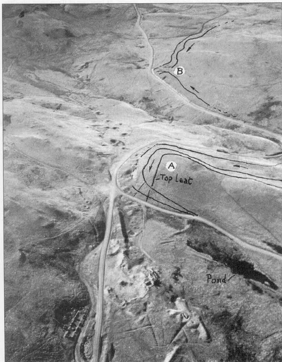
Fig. 1. An aerial view of Esgairhir taken by the Royal Commission on Historical Monuments (Wales), with the six leats inked in. Three skirt the ridge at A, and three converge at trial workings at B. The main lode runs from top to bottom of the picture.
