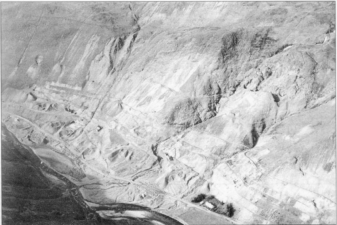
Fig. 6. Aerial view of the western part of the Cwmystwyth Mine. Prospecting Hushes are clearly visible descending the hillside to the top left and on every other piece of upland green pasture above the mine. The great opencasts on the Graig Fawr can be seen towards the top right with the dense complex of hushing channels descending from the waterfall above. (Crown copyright, Royal Commission on the Ancient and Historical Monuments of Wales).
