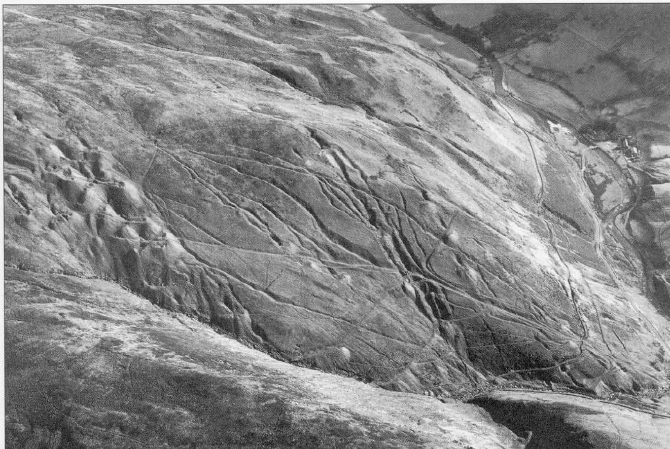
Fig. 2. Hushing channels on Copa Hill, the deepest (with the Bronze Age opencast at top) are on the centre-right. To the left of these deep gashes are a shallower series radiating from a supply pond to the top-left which itself cuts an earlier leat leading to the head of the deep channels near the early opencast. (Crown copyright, Royal Commission on the Ancient and Historical Monuments in Wales).
